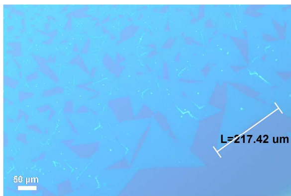
Figure S1: The optical image of CVD grown 1L-MoS 2 .
